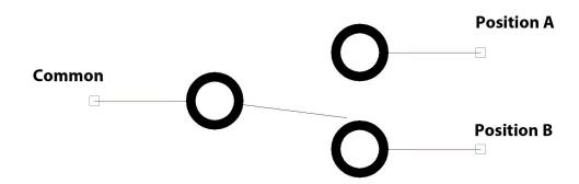
This push button switch is a push-on push-on type (Either Or). It mounts in a 15/32" hole and includes mounting nuts and washers and an attractive chrome cap. The thread length is 1/2"
